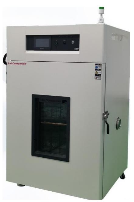
Our large-capacity high-temperature industrial ovens can be customized with various optional functions, sizes/indicators/capacity, etc. according to user requirements. The maximum temperature limit optional 300°C.
